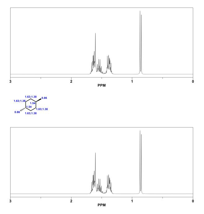
There does not seem to be much of a difference between these two spectra. However, notice that the compounds are diastereomers (see below), and as such, you should not expect the spectra to be perfectly superimposable.
