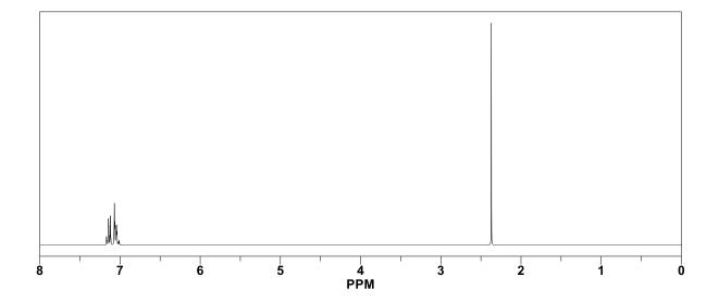
The spectrum contains a singlet for the CH<sub>3</sub> (around 2 ppm, CH<sub>3</sub> linked to aromatic).
