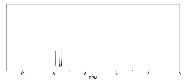
The <sup>1</sup>N NMR spectrum shows 1 peak around 10 ppm. This is very characteristic of aldehydes: we have a **CHO**-group. This also explains the 2700-3100 cm<sup>-1</sup> absorption in the IR, it is the aldehyde's C-H.
