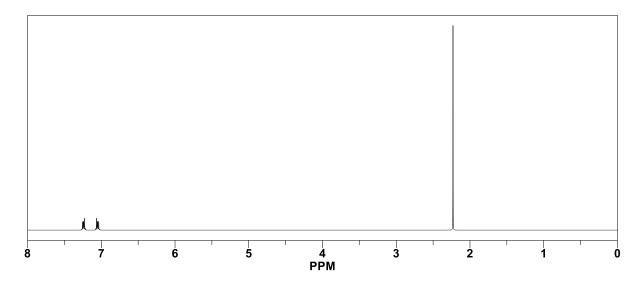
The compound is symmetric, so there is one signal for the methyls (integration 3 (or 6)), one for the aromatic C-H's next to the methyl (7.24 ppm, doublet integration 1 (or 2)), and one for the aromatic C-H further from the  $CH_3$  (7.05 ppm, doublet, integration 1 (or 2) – this is only split by the non-identical hydrogen, and not the one that is identical to itself!).
