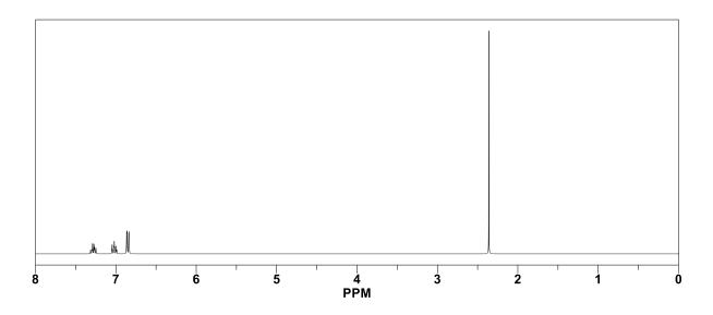
There are a couple of things about this one. First of all, hydrogens can couple to fluorines (don't think it came up in the lectures), so the C-H signals of the H neighboring the C-F are split by the F. Also, it is only a coincidence that there are two signals that are both at 6.85 ppm, because the hydrogens that give rise to them are obviously not identical. One is between a methyl and a C-F, the other between a methyl and a C-H.
