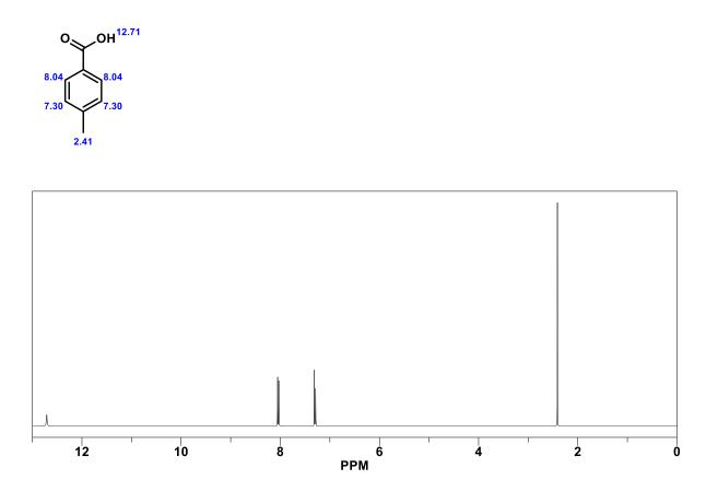
The compound is symmetric. It has a COO<u>H</u> signal, which is usually around 11-12 ppm. You might also see that it is a bit broader than the other signals, which is typical of OH, NH, SH-signals. The aromatic region contains two signals, each of integration 2 (doublets, have 1 neighbor each that is not identical to them). Finally, there is a singlet for the aromatic-linked C<u>H</u><sub>3</sub> group.
