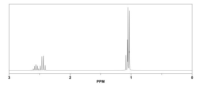
The methyls of the isopropyl group are identical, integrating to 6. They are split to a doublet by the C-H. The C-H itself is integration 1, split to a septet by the 6 identical hydrogens in the two methyl groups.
